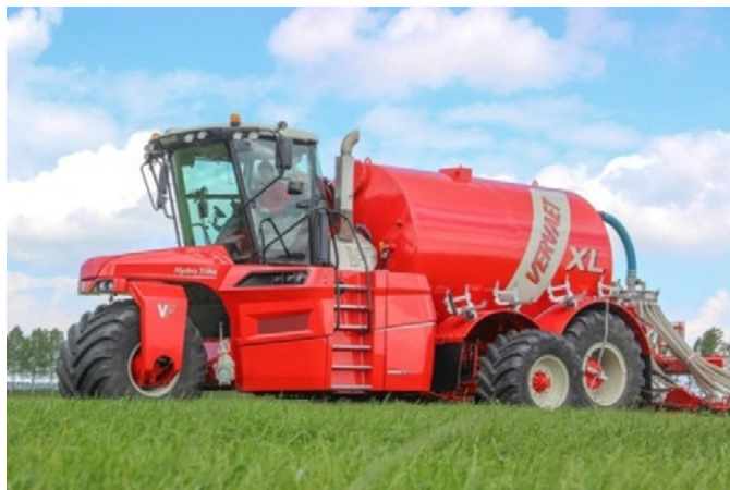
Figure 7: Precision manure tank equipped with nutrient sensing technology
